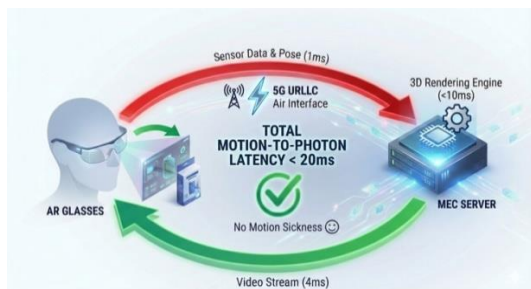
Fig 2: A Private 5G Network Deployed With Edge Applications on an MEC Server to Support Augmented Reality
