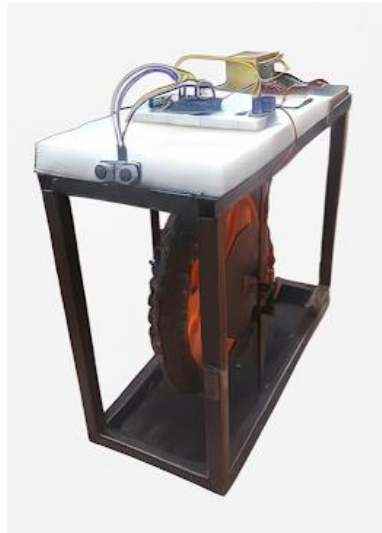
Fig 1: AI-Assisted Automated Electromagnetic Braking System Prototype (Arduino-Based)
