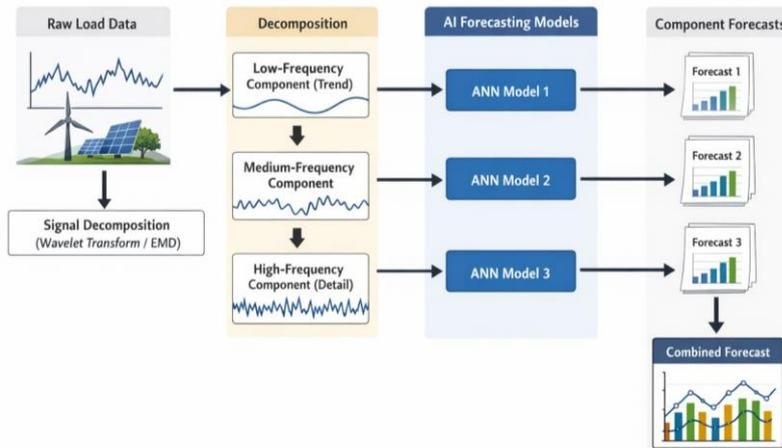
**Fig 4: Hybrid Load Forecasting Framework Combining Decomposition and AI**
